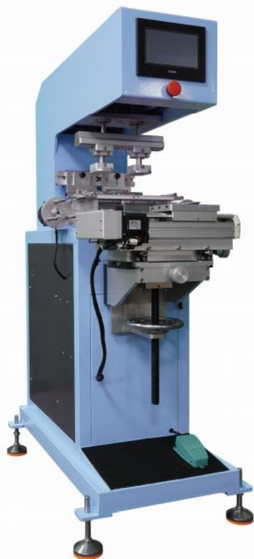
Full Electric Two Color Closed Ink Cup Pad Printer with Shuttle Work Table and Automatic Pad Cleaning System 电动双色移印机 (自动清洁系统)
