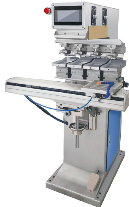
P4/S四色穿梭伺服 P4/S Four colors servo with shuttle
